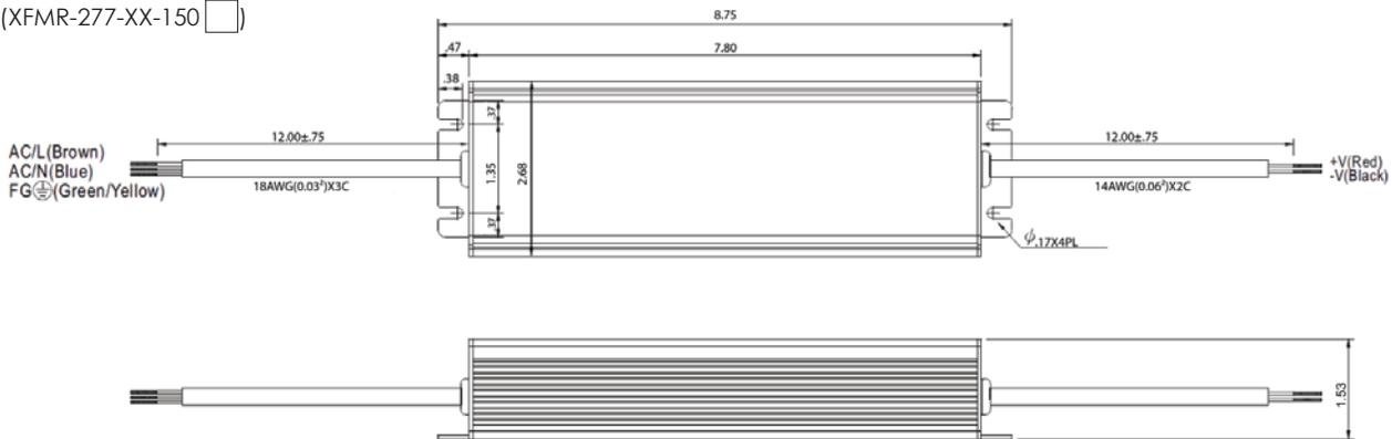
※IP67 rated. Cable for I/O connection.
