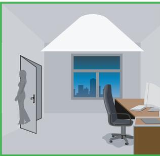
The light dims to stand-by period after hold-time and stays on at the selected minimum dimming level.
