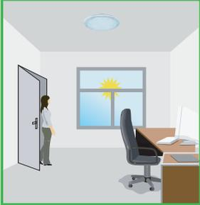
The light will not switch on when natural light is sufficient, even when there is motion detected.
