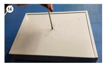
13. Remove any burrs from the hole (if necessary) and insert the plastic grommet. (Fig. 15 and 16)
