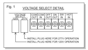
**CAUTION:** Failure to install the Voltage Selector Plug will prevent system operation. Installing the Voltage Selector Plug in the position that does not match the actual AC input line voltage will damage the unit, void the warranty, and may cause a dangerous or unsafe condition.
