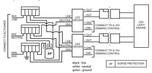
4: Connect the LED driver harness(s) to the LED light engine.
