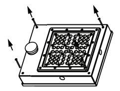
2: Mount cover plate to junction box using the provided slots. Use appropriate hardware for application.
