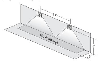
Using multiple units mounted at a typical 8' delivers 20' center-to-center spacing on a 6' wide egress path.
