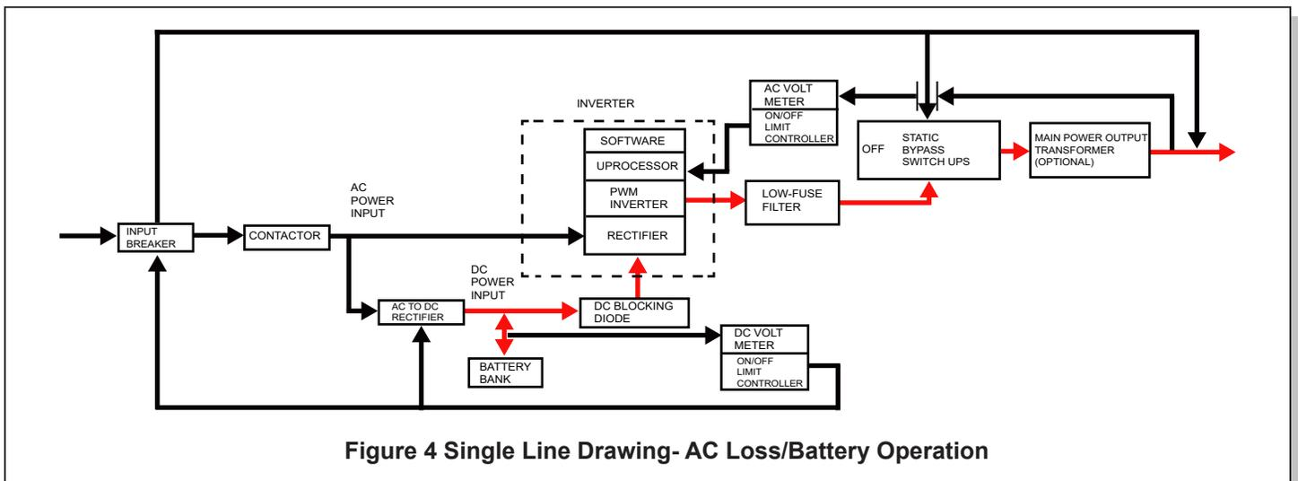
Figure 4 Single Line Drawing- AC Loss/Battery Operation
