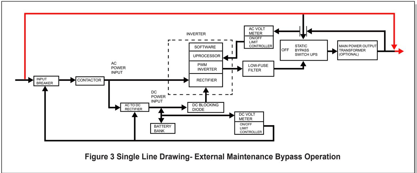
Figure 3 Single Line Drawing- External Maintenance Bypass Operation
