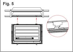
Align the hooks on the panel with the slots on the mounting brackets, hook them onto the brackets for side-mounted installation ensuring a tight grip. (Fig. 5)
