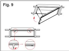
Rotate the panel upwards and push into the original housing. Push the rotary clips to secure the panel until a "click" sound is heard. Installation is now complete. (Fig. 9)
