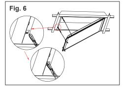
Hook each of the safety wires to the hole of the mounting bracket to suspend the panel body. (Fig. 6)
