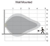
Highest mounting height is 4m This figure indicates the maximum distance at the highest mounting height with 100% sensitivity.
