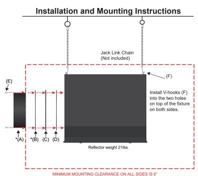
\*When installing fixture only use either the included (A) 8" removable flange or (B) louvered plate or (C) closed off plate with (E) thumbscrews and (D) 8" silicone seal (Do not use all in combination).
