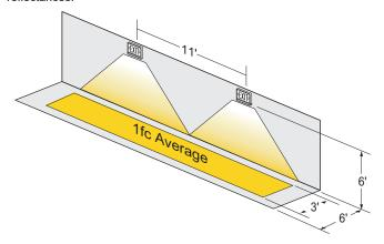
Using multiple LOBO units mounted at a typical 6' height delivers 10' on-center spacing with a 6' wide path of egress using 80/50/20 reflectances.
