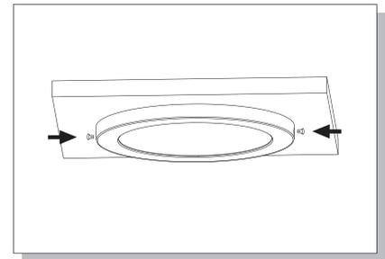
3. Align the light slots with the mounting bracket slots and secure with plastic push-in clips. Press light flush with surface and install optional magnetic trim ring if compatible.
