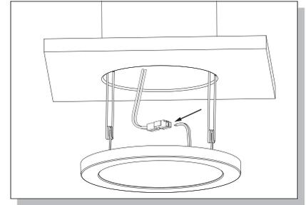
6. Insert wires into adapter connector per wiring diagram. Set color switch if equipped.
