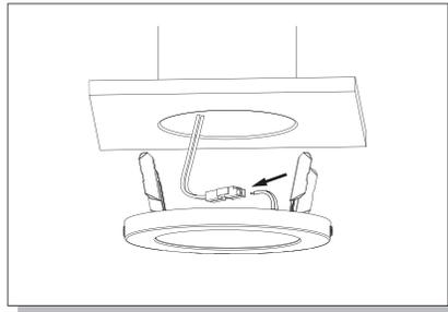
4. Insert light wires into adapter connector, make wiring connections per wiring diagram. Set color switch if equipped.
