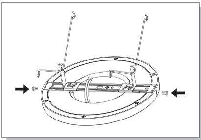
4. Install light to mounting bracket and secure with plastic push-in clips.
