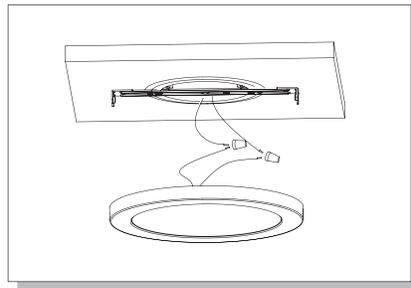
2. Make wire connections (see Wiring diagram). Set color switch if equipped.
