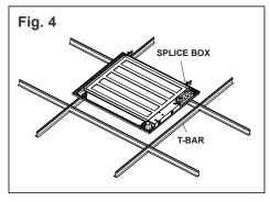
4. Place the luminaire on the T-bar of the ceiling suspension system in the desired location. (Fig. 4)
