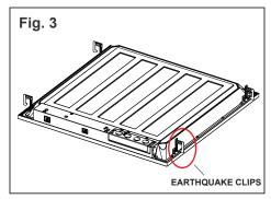
3. Locate all four earthquake clips on the back of the luminaire. Twist each tab away from the luminaire and test them on the T-bar. (Fig. 3)
