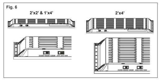
6. Select the CCT and wattage you need by adjusting the switches on the side of the connection box. (Fig. 6)
