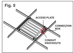
5. Open the fixture J-box by removing the access plate and make electrical connections. (Fig. 5 and Electrical Connections section). Make sure to firmly secure conduit to the access plate before replacing the access plate to the fixture J-box when complete.
